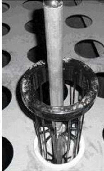
Pic. 2. Filter bag “Ad-flow” with the cage
