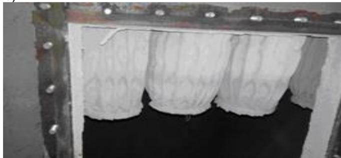
The Pic. 9. Filer bag 3DESA patron in production of the dry mixtures
