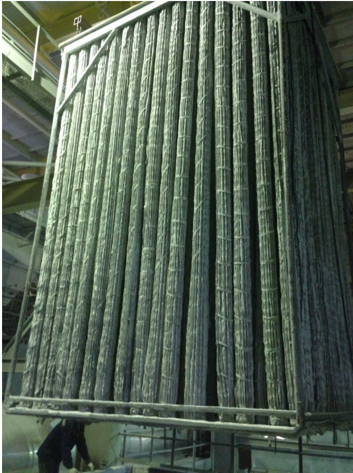
Fig. 13. Montage of the filter bags "3DESA filtratron"
